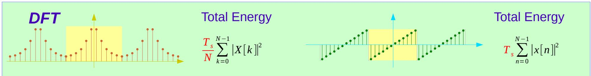
$$X(jk\omega_0) \approx T_s X[k] \quad \frac{1}{2\pi} \int_{-\infty}^{+\infty} |X(j\omega)|^2 d\omega \quad \longrightarrow \quad \frac{1}{NT_s} \sum_{k=0}^{N-1} |T_s X[k]|^2 = T_s \sum_{n=0}^{N-1} |x[n]|^2 \quad \longleftarrow \quad \int_{-\infty}^{+\infty} |x(t)|^2 dt$$
