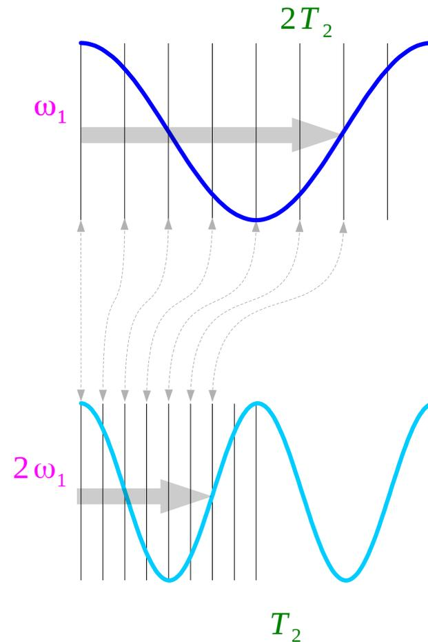
$$f_0 n = \text{const}, n T_s = \text{const}$$
