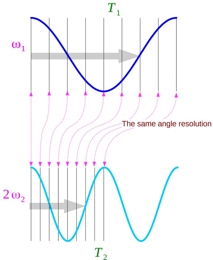
$$\theta_1 = \omega_1 t_1 = \omega_1 n T_1 = \Omega_1 n$$
