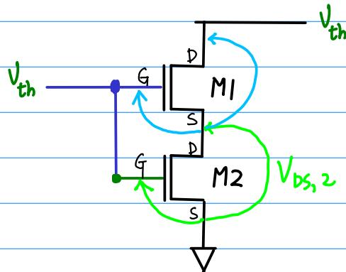
$$\begin{aligned} V_{th} &= V_{GS1} + V_{DS2} \\ &= V_{GS2} \end{aligned}$$
