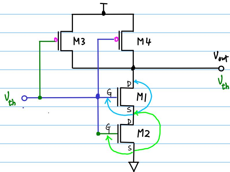
$$M_1 \text{ SAT} \quad I_D = \frac{B_0}{2} (V_{th} - V_{Ton} - V_{DS,2})^2$$
