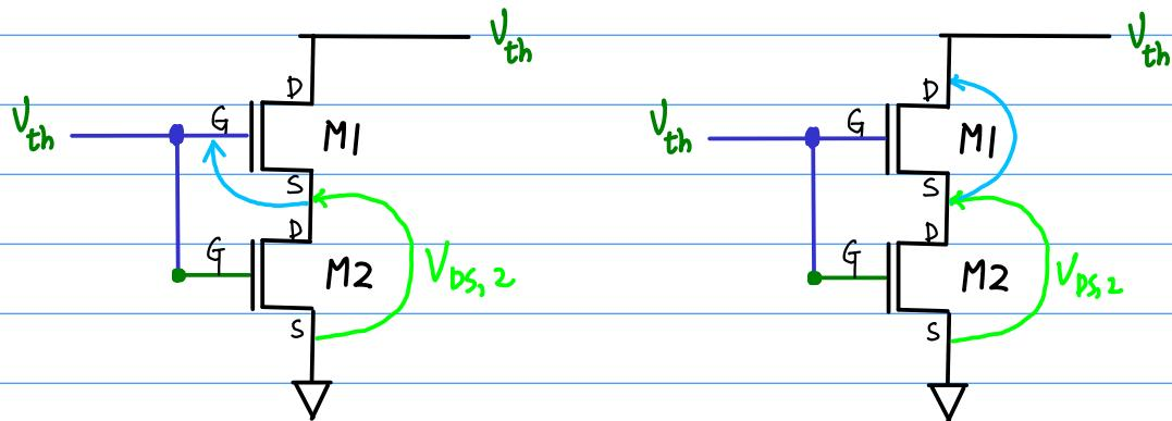
$$V_{GS,1} = V_{th} - V_{DS,2}$$
