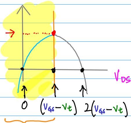
$$V_{DS} \leq V_{GS} - V_t$$
