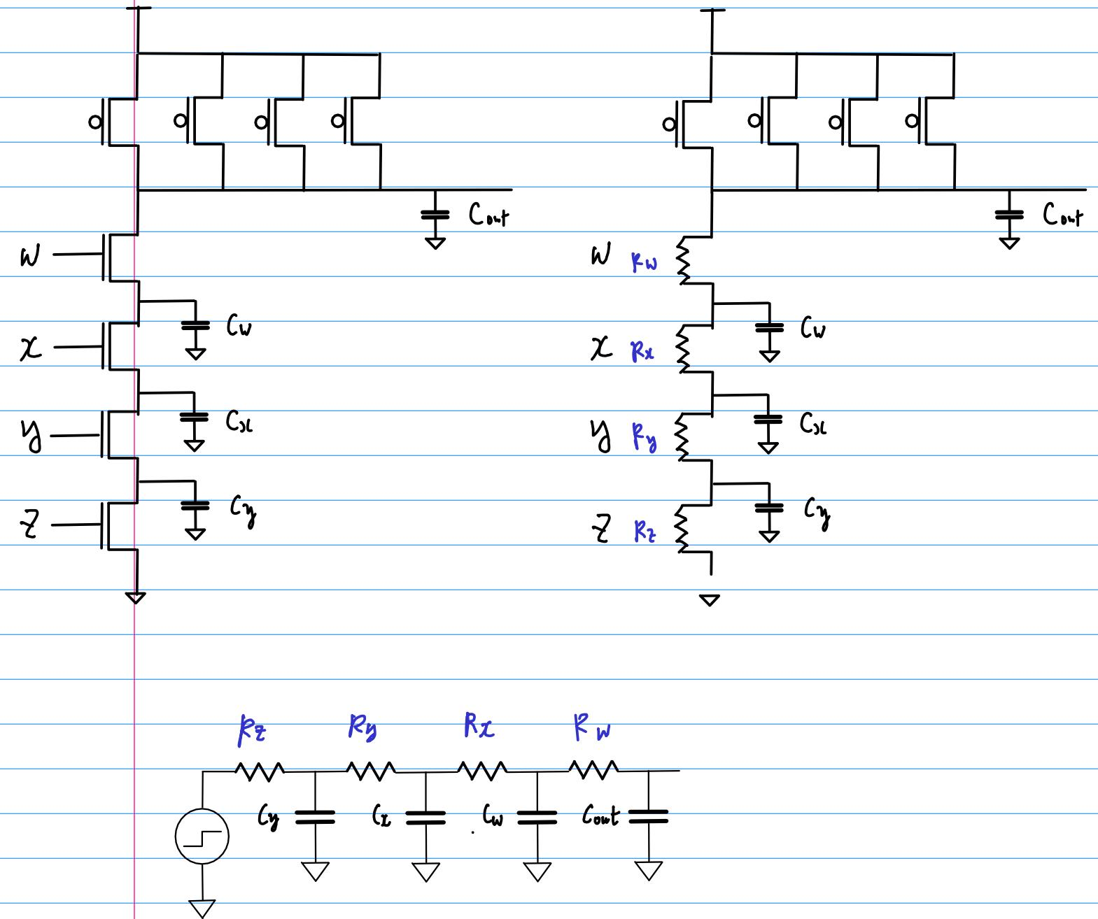
$$t_{pd} = C_y R_z + G_x (R_y + R_z) + C_w (R_x + R_y + R_z) + C_{out} (R_w + R_x + R_y + R_z)$$
