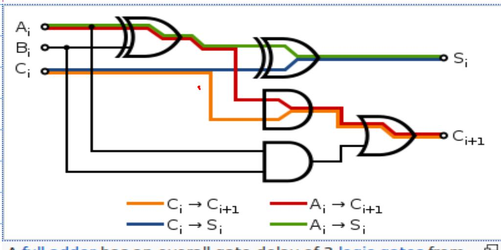
A full adder has an overall gate delay of 3 logic gates from the inputs  $A$  and  $B$  to the carry output  $C_{\text{out}}$  shown in red
