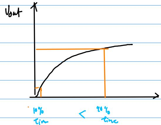
$$i = -C_{out} \frac{dV_{out}}{dt} = \frac{V_{pp} - V_{out}}{R_p}$$
