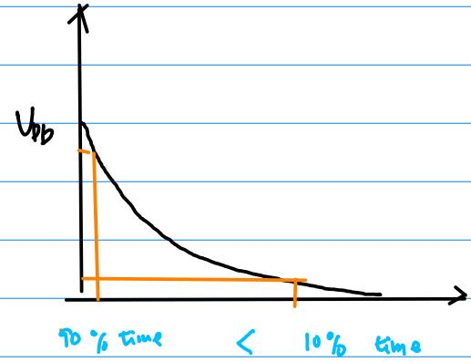
$$i = -C_{out} \frac{dV_{out}}{dt} = \frac{V_{out}}{R_n}$$
