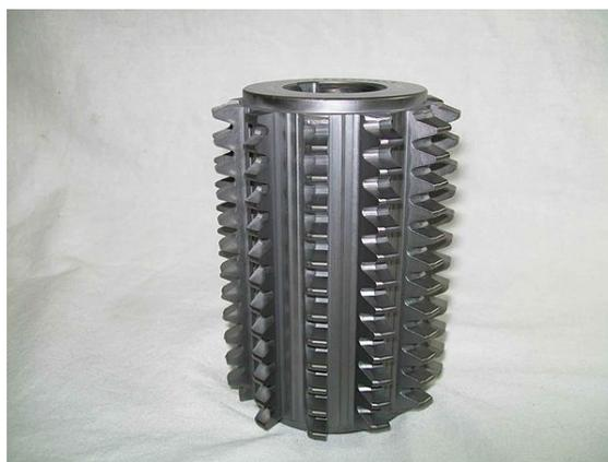
*Aluminium Chromium Titanium Nitride (AlCrTiN) coated Hob using Cathodic arc deposition technique*
