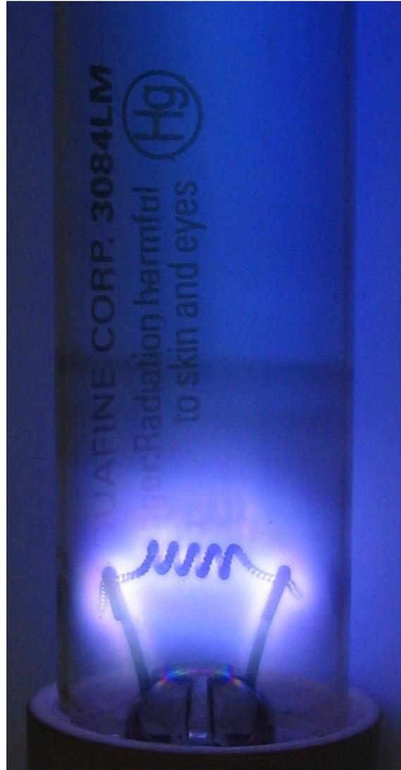
*The unfiltered ultraviolet glow of a germicidal lamp is produced by a low pressure mercury vapor discharge (identical to that in a fluorescent lamp) in an uncoated fused quartz envelope.*
