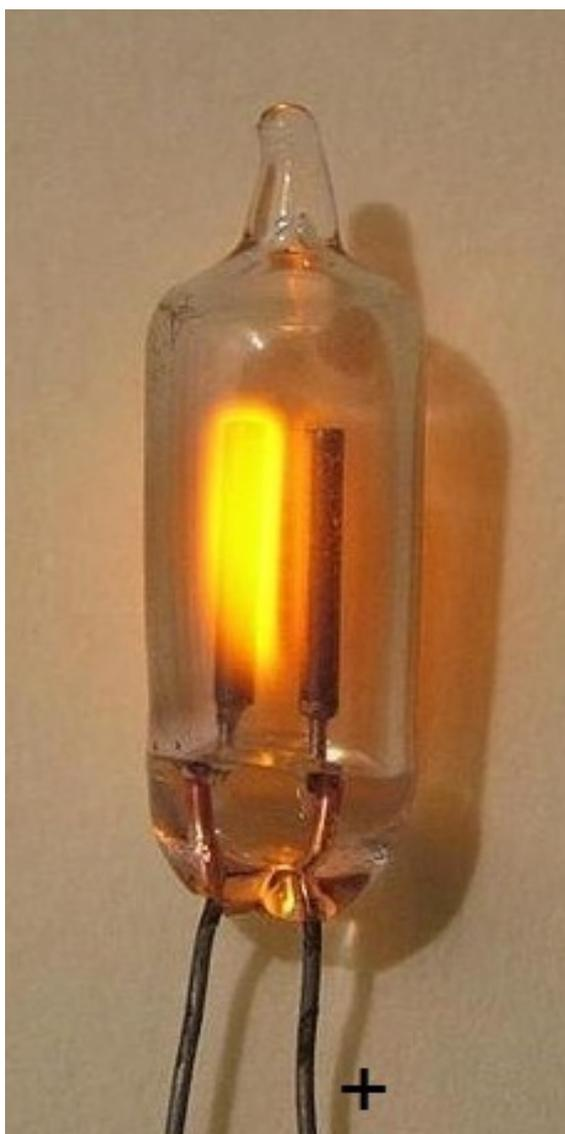
Neon lamp, 1/2 inch, showing glow discharge surrounding cathode.
