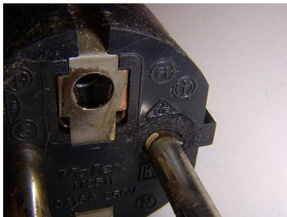
*Arc damage to a CEE 7/7 plug. The discharge path was formed by a conductive liquid seeping into the plug-socket assembly.*
