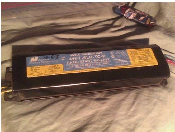
A rapid-start “iron” (magnetic) ballast continually heats the cathodes at the ends of the lamps. This ballast runs two F40T12 lamps in series.
