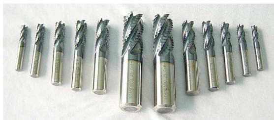
*Aluminium Titanium Nitride (AlTiN) coated endmills using Cathodic arc deposition technique*
