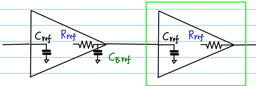
$$p = \frac{z_{par}}{z} = \left( \frac{k R_{ref} C_{p,ref}}{k R_{ref} C_{ref}} \right) = \left( \frac{C_{p,ref}}{C_{ref}} \right)$$
