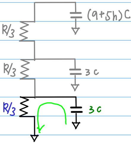
$$\begin{aligned} & (R/3)(3C) \\ & = RC \end{aligned}$$
