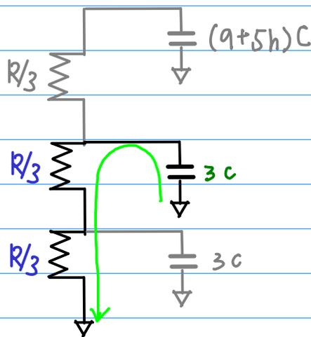
$$\begin{aligned} & (R/3 + R/3)(3C) \\ & = 2RC \end{aligned}$$
