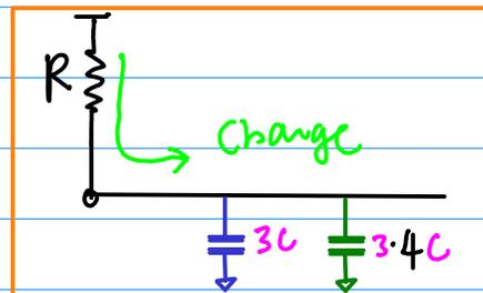
$$\begin{aligned}t_{pd} &= (R)(3C + 3.4C) \\ &= (3 + 3.4)RC \\ &= 3RC(1 + 4) \\ &= \tau(1 + 4)\end{aligned}$$
