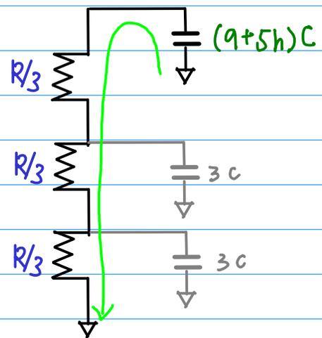
$$\begin{aligned} & (R/3 + R/3 + R/3)(9+5h)C \\ & = (9+5h)RC \end{aligned}$$
