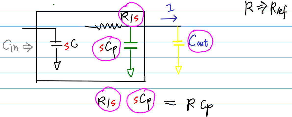
$$P = \left( \frac{C_{p,ref}}{C_{ref}} \right) = \left( \frac{\text{internal diffusion cap.}}{\text{gate cap of ref inv}} \right)$$
