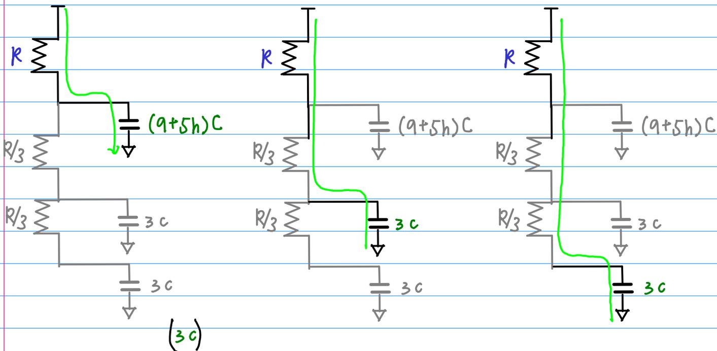
$$\begin{aligned} & (R)(9+5h)C \\ & = (9+5h)RC \end{aligned}$$
