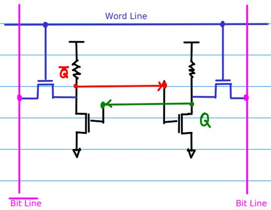
resistor & redundant tr removed
