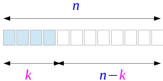
$$\begin{aligned} P(n, k) &= \frac{n!}{(n - k)!} \\ &= (n-0) \cdot (n-1) \cdot (n-2) \cdots (n-(k-1)) \end{aligned}$$
