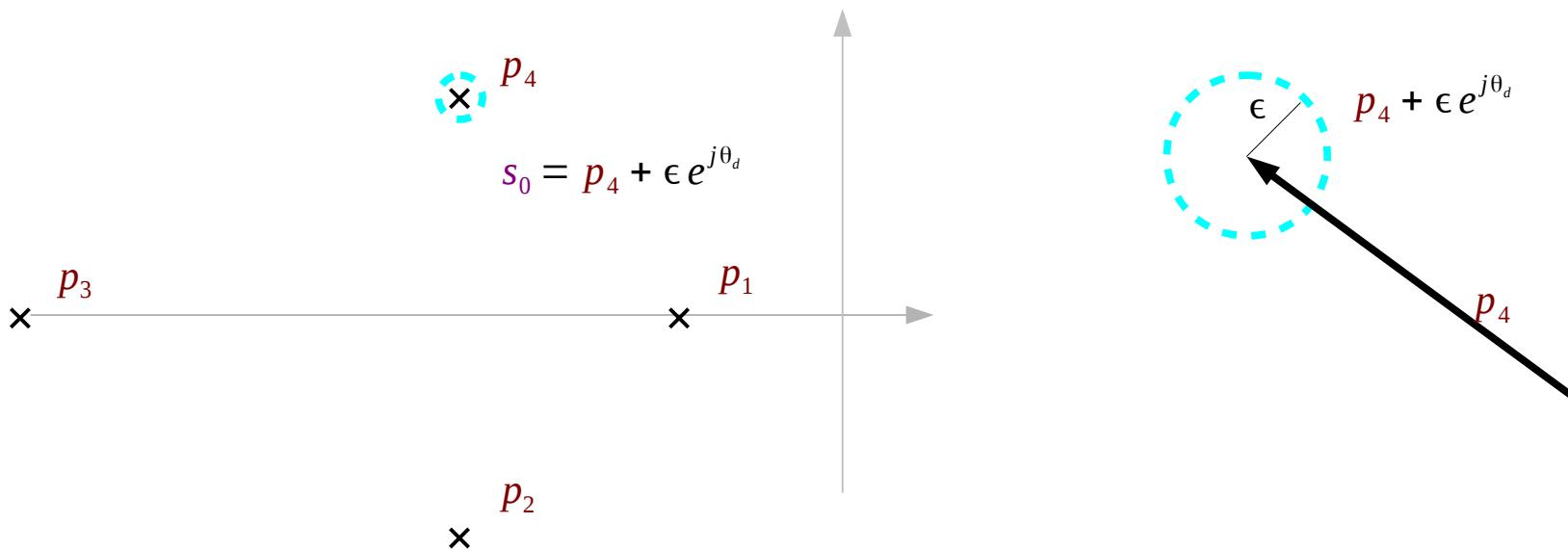
$$\arg(s_0 - z_1) + \arg(s_0 - z_2) + \cdots + \arg(s_0 - z_m) - [\arg(s_{0s} - p_1) + \arg(s_0 - p_2) + \cdots + \arg(s_0 - p_n)] = (2q+1)\pi \quad K > 0 \quad \text{positive root locus}$$
