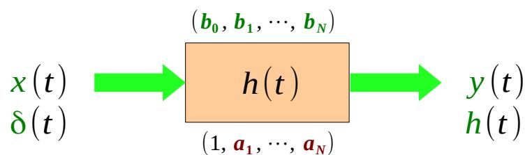
$$y(t) = b_N w(t) + b_{N-1} w^{(1)}(t) + \dots + b_0 w^{(N)}(t)$$
