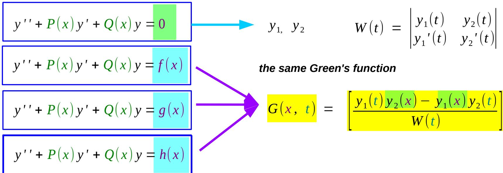
$$y_p = u_1(x)y_1 + u_2(x)y_2 = \int_{x_0}^x G(x, t)f(t)dt = \int_{x_0}^x \left[ \frac{y_1(t)y_2(x) - y_1(x)y_2(t)}{W(t)} \right] f(t)dt$$
