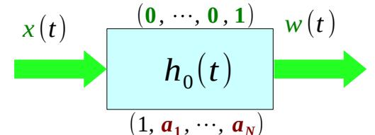
$$\left. \begin{array}{l} b_N \left[ \begin{array}{c} w^{(N)} \\ w^{(N-1)} \\ \vdots \\ w^{(2N)} \end{array} \right] + a_1 \left[ \begin{array}{c} w^{(N-1)} \\ w^{(N)} \\ \vdots \\ w^{(2N-1)} \end{array} \right] + \cdots + a_{N-1} \left[ \begin{array}{c} w^{(1)} \\ w^{(2)} \\ \vdots \\ w^{(N+1)} \end{array} \right] + a_N \left[ \begin{array}{c} w \\ w^{(1)} \\ \vdots \\ w^{(N)} \end{array} \right] = x \end{array} \right\} 0$$
