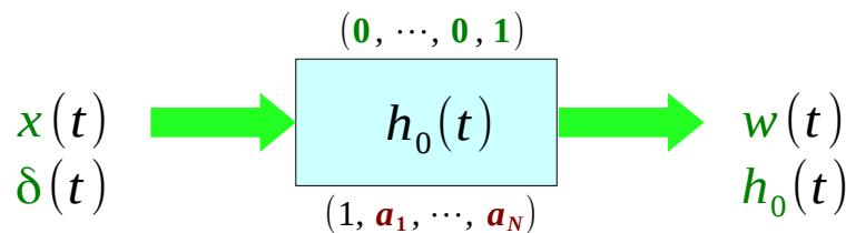
$$\begin{aligned} Q(D)w(t) &= x(t) \\ Q(D)h_0(t) &= \delta(t) \end{aligned}$$
