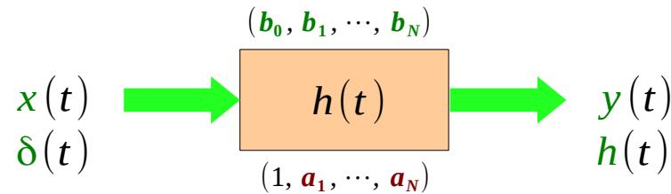
$$y = b_0 w^{(N)} + b_1 w^{(N-1)} + \dots + b_N w$$
