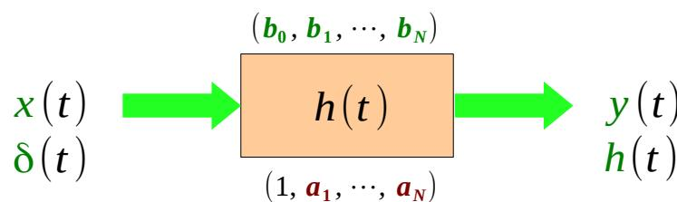
$$\begin{aligned} Q(D)y(t) &= P(D)x(t) \\ Q(D)h(t) &= P(D)\delta(t) \end{aligned}$$
