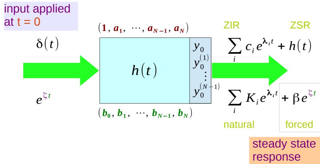
$$\begin{array}{|c|} \hline x(t) = A \\ \xi = 0 \\ \hline \end{array} \rightarrow \begin{array}{|c|} \hline h(t) \\ \begin{bmatrix} y_0 \\ y_0^{(1)} \\ \vdots \\ y_0^{(N-1)} \end{bmatrix} \\ \hline \end{array} \rightarrow \begin{array}{|c|} \hline y_{ss}(t) = H(0) \cdot A e^{0t} \\ = A \cdot H(0) \\ \hline \end{array}$$
