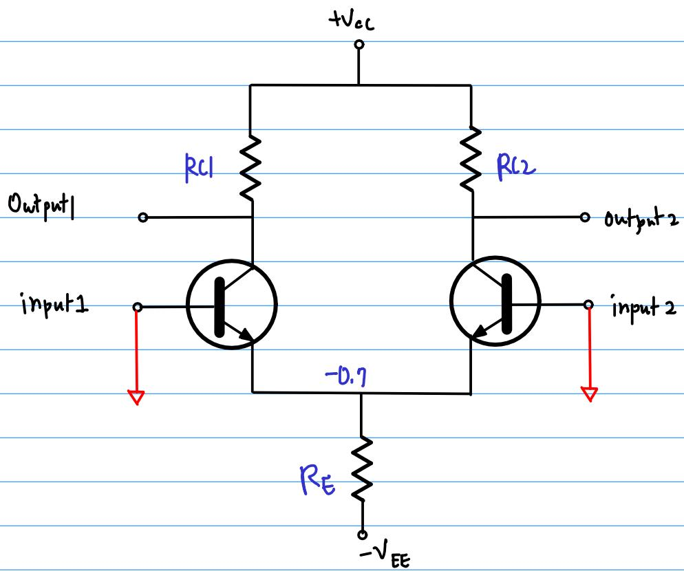
Bias on input 1 and ground on input 2
