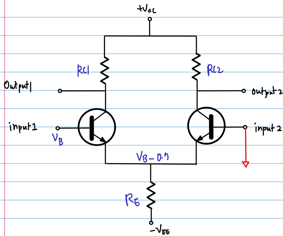
Ground on input2 and bias on input1
