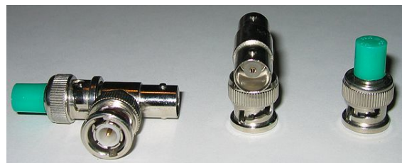
BNC Tee Connectors with resistive load terminators
