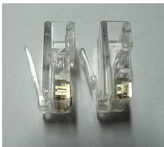
8P8C plug with contacts for solid wire (left) and stranded wire (right)
