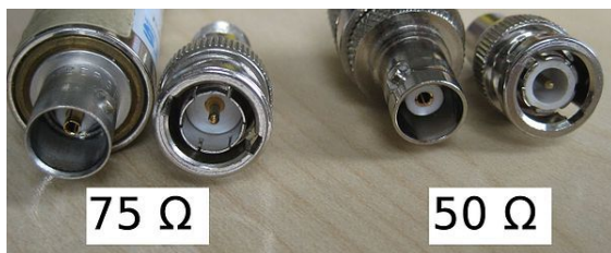
BNC connectors. From left to right: 75 Ω female, 75 Ω male, 50 Ω female, 50 Ω male.
