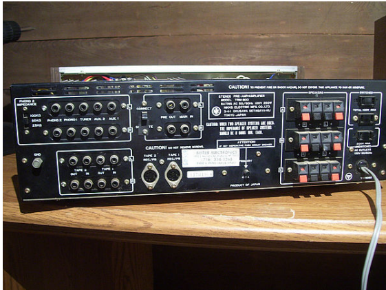
Back of an audio power amplifier features a variety of electrical connectors
