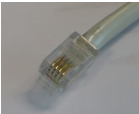
4P4C modular connector on a handset cord
