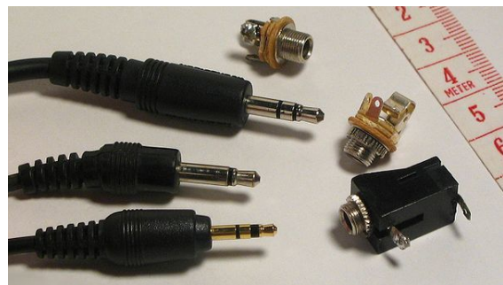
Miniature phone plugs and jacks. All are 3.5 mm except the gold-plated plug, which is 2.5 mm. One of the 3.5 mm jacks is two-conductor and the others are three conductor. The tan-colored jacks have a normally-closed switch.
