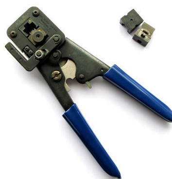
A modular plug crimper
