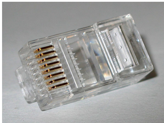
An 8P8C modular plug before being crimped onto a cable
