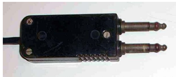
A dual 310 patch cable, two-pin phone plug
