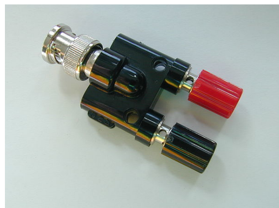
A binding post (red and black) adaptor.
