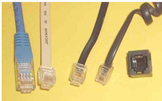
Left to right, modular connectors: 8P8C plug, 6P6C plug, 6P4C plug, 4P4C plug, 6P6C jack.
