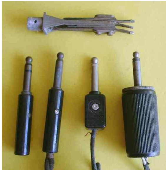
Old-style male tip-sleeve (“pin” or “jack”) connectors. The left-most plug has three conductors; the others have two. At the top is a three-conductor jack from the same era.
