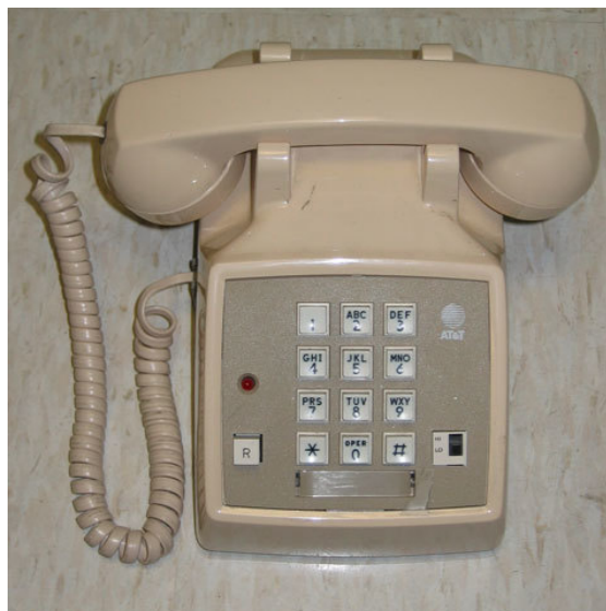
Wired telephone that uses 4P4C connectors for the coiled handset cord
