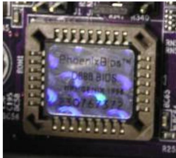
PhoenixBIOS D686. This BIOS chip is housed in a PLCC package in a socket.
