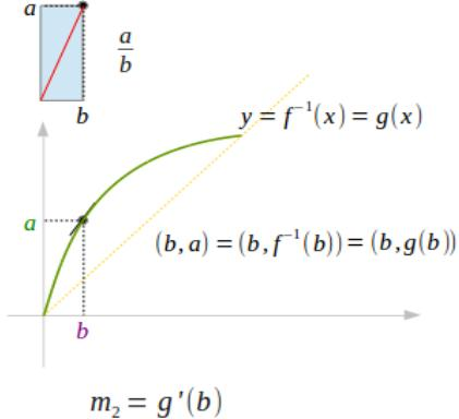
$$m_1 m_2 = f'(\text{a}) g'(\text{b}) = 1 \Rightarrow g'(\text{b}) = \frac{1}{f'(\text{a})} \Rightarrow g'(\text{b}) = \frac{1}{f'(g(\text{b}))}$$
