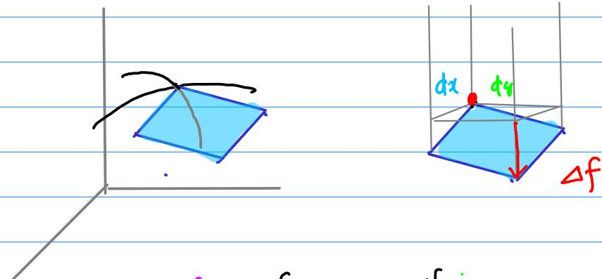
total differential  $df = \frac{\partial f}{\partial x} dx + \frac{\partial f}{\partial y} dy \quad \dots \quad \mathbb{R}^3, z = f(x, y)$
