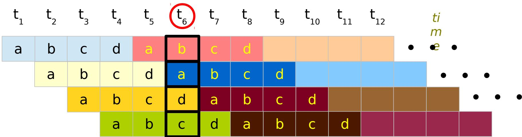
The subtask snapshot at time  $t_6$
