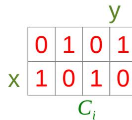
$$S = \bar{x}\bar{y}C_i + \bar{x}y\bar{C}_i + x\bar{y}\bar{C}_i + xyC_i$$
