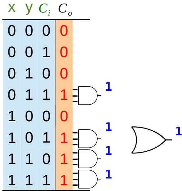
$$C_o = \bar{x}yC_i + x\bar{y}C_i + xy\bar{C}_i + xyC_i$$
