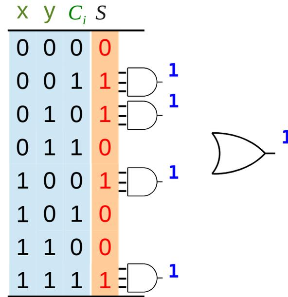
$$S = \bar{x}\bar{y}C_i + \bar{x}y\bar{C}_i + x\bar{y}\bar{C}_i + xyC_i$$
